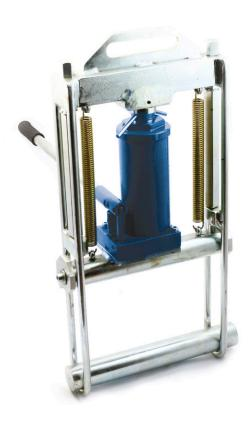
The hydraulic pipe squeeze-off tool is used for emergency, temporary shutting off the flow in polyethylene gas and water pipelines. The squeezing force is generated by a hydraulic cylinder driven manually by a lever.
